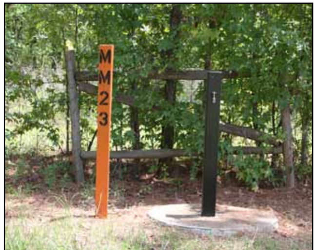
Methane Monitoring Well
